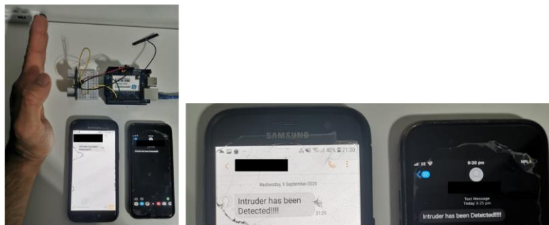
Fig. 6. SMS Intruder alert sent to the recipients’ mobile phones successfully in real-time on the left-hand side of the figure and a clearer view of SMS sent on the right-hand side of the figure.
