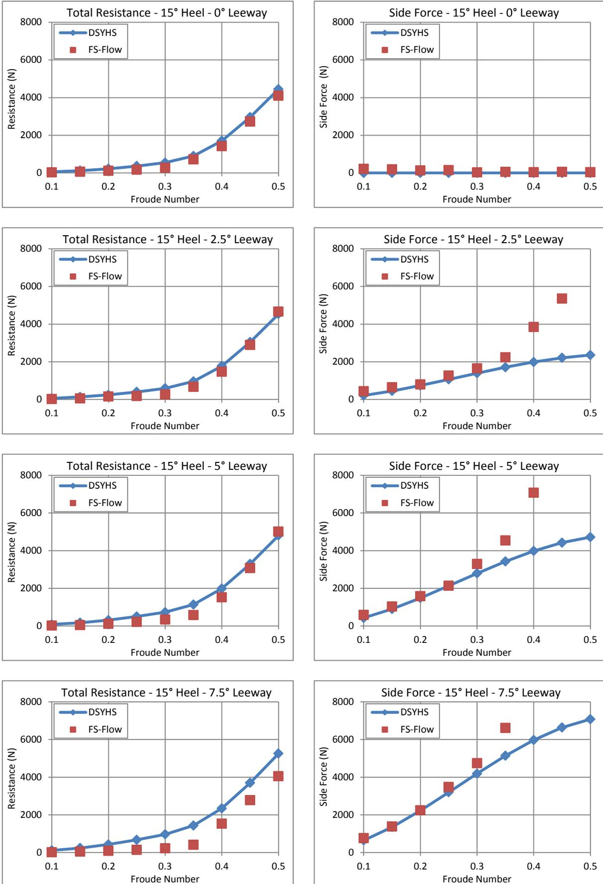
Figure 52: Stewart 34 hydrodynamic model: FS-Flow and DSYHS comparison, 15° Heel.
