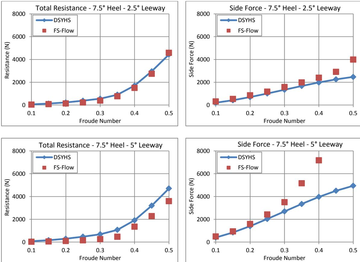
**Figure 28:** Typical example of FS-Flow results for the hydrodynamic model of the Stewart 34.
