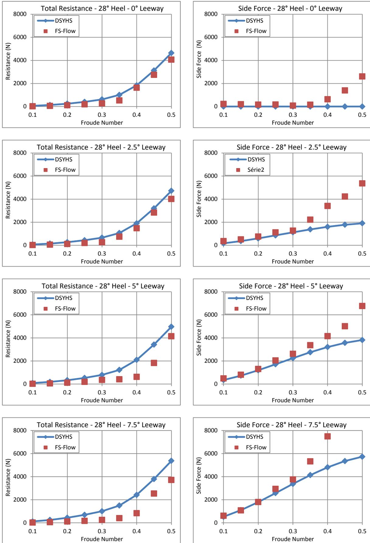
Figure 54: Stewart 34 hydrodynamic model: FS-Flow and DSYHS comparison, 28° Heel.
