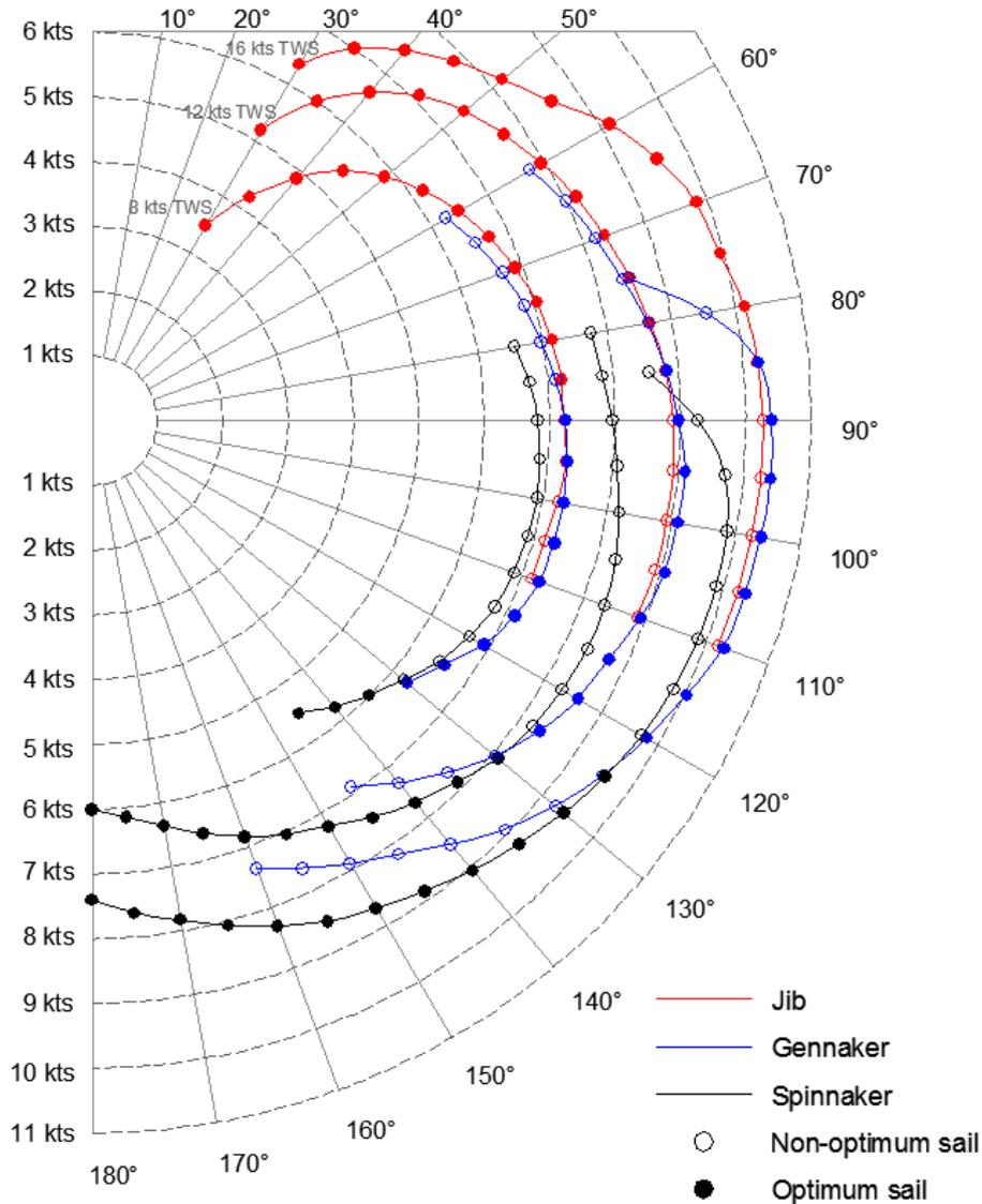
**Figure 33:** *Fs-Equilibrium VPP, boat speed (knots).*
