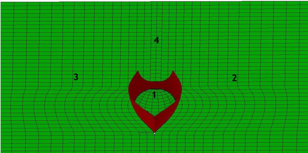
**Figure 15:** Sysser 62 meshing (exaggerated for clarity) realised in FS-Flow.
