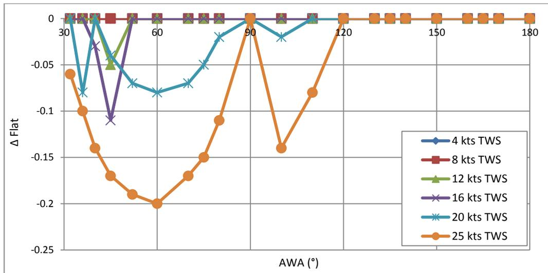
**Figure 65:** Flat difference between FS-Equilibrium and WinDesign.
