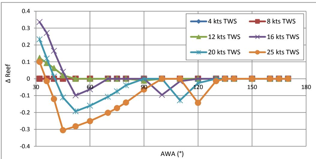
**Figure 64:** Reef difference between FS-Equilibrium and WinDesign.
