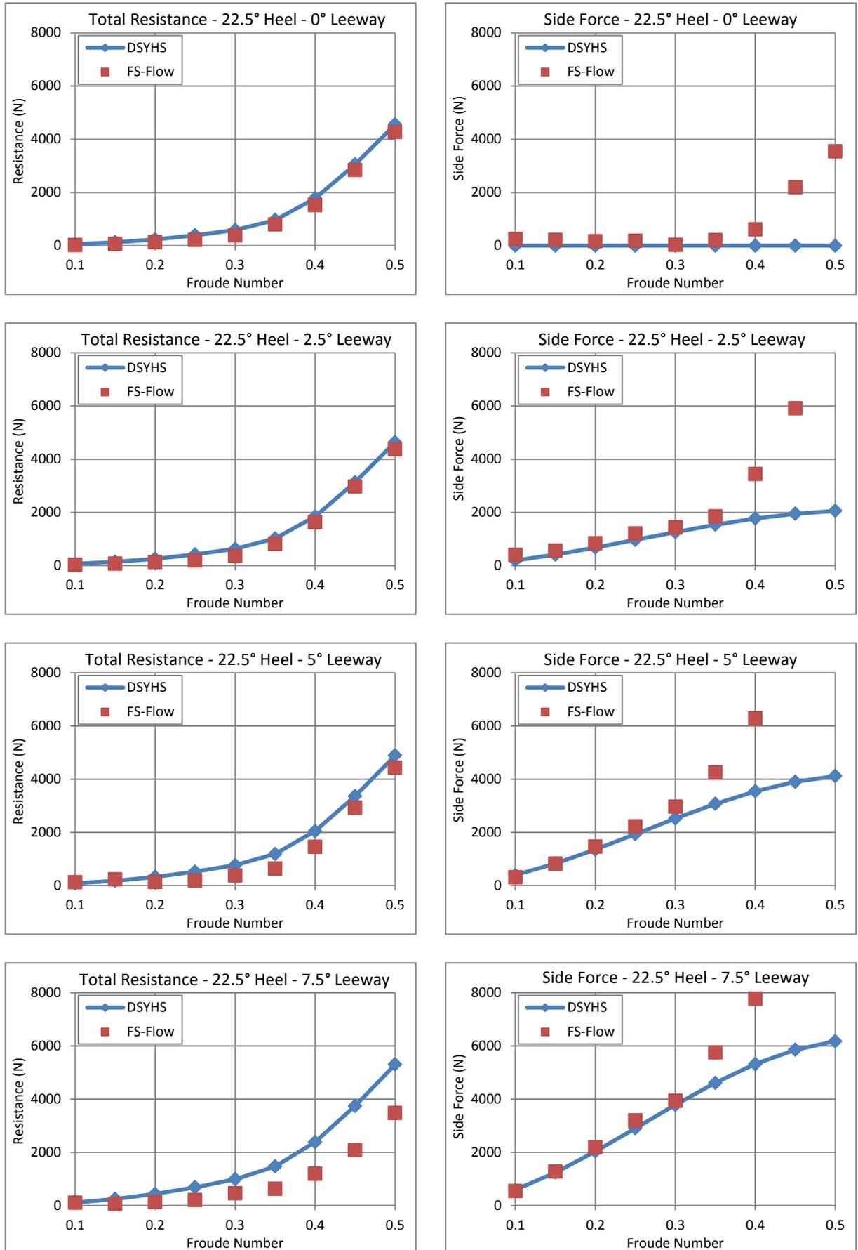
**Figure 53:** Stewart 34 hydrodynamic model: FS-Flow and DSYHS comparison, 22.5° Heel.
