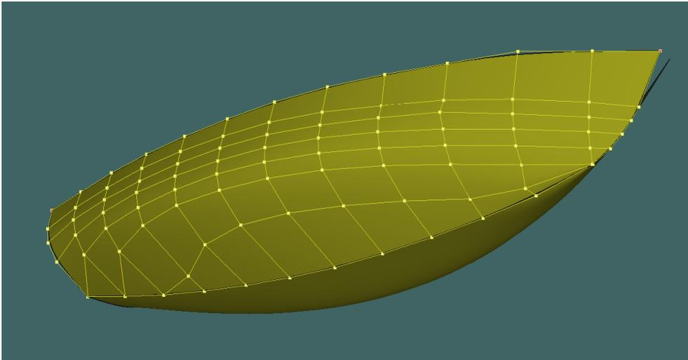
**Figure 48:** Additional waterline added to the model of the Stewart 34.
