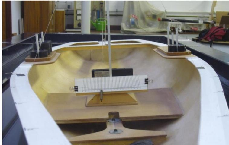
**Figure 57:** Model scale inclining experiment illustrating a typical setup.
