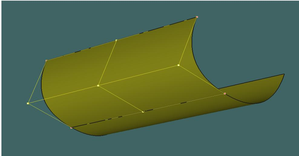
**Figure 45:** Half cylinder, starting point of the 3D lofting.
