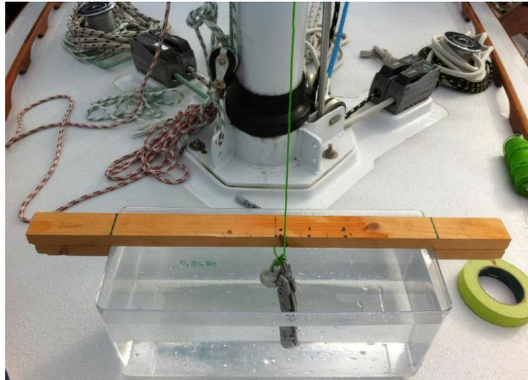
**Figure 58:** Pendulum setup for the inclining experiment of the Stewart 34, illustration from [79].
