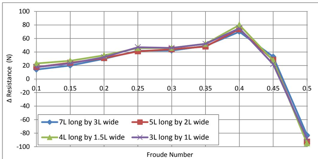
**Figure 18:** Impact of the domain size on the resistance ( $\Delta x=0.05$ ).
