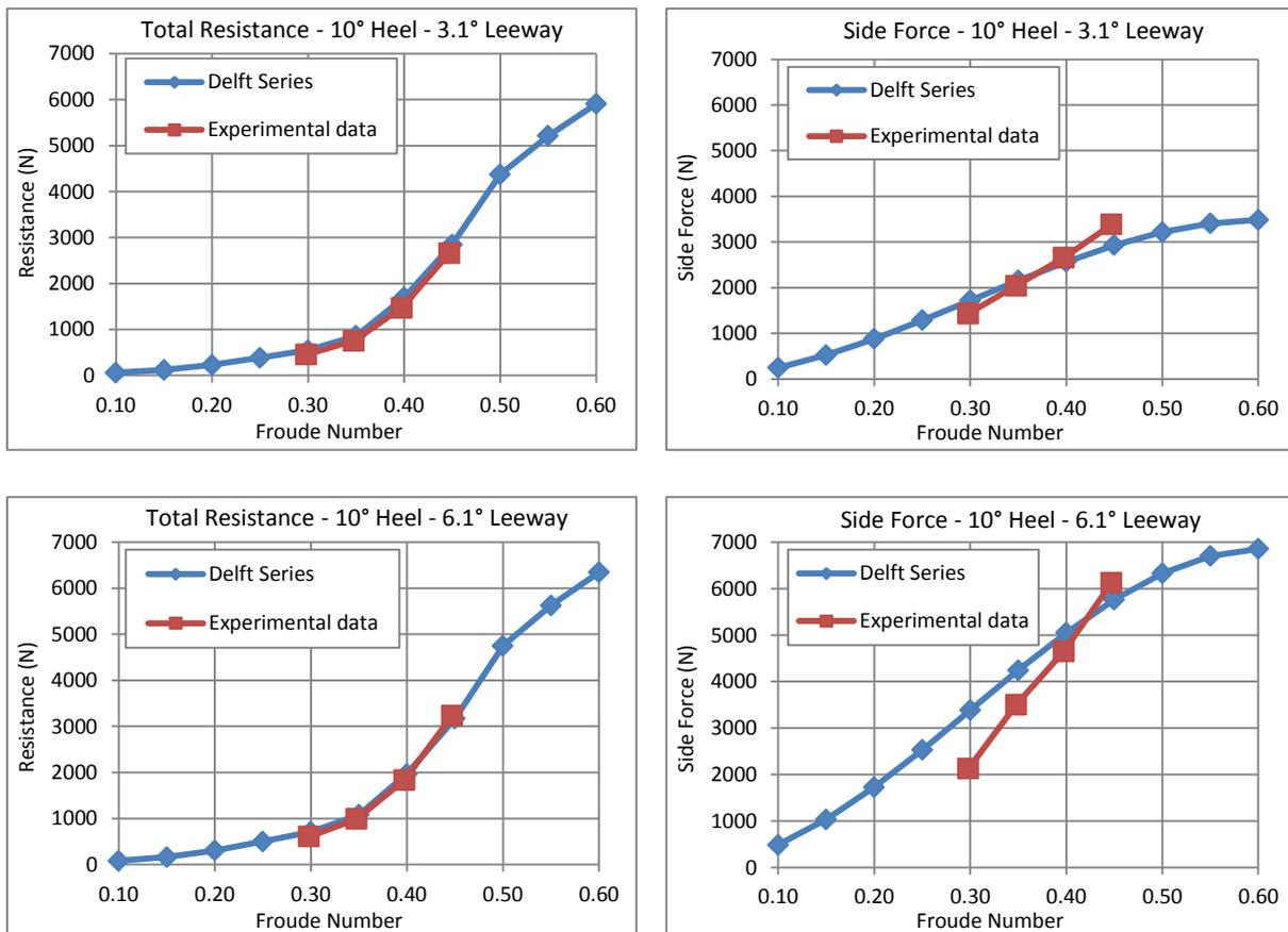
Figure 9: DSYHS and experimental data [18] comparison at 10° of heel.
