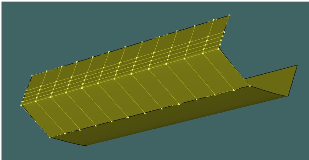
**Figure 46:** Surface net matching the tables of offsets grid.
