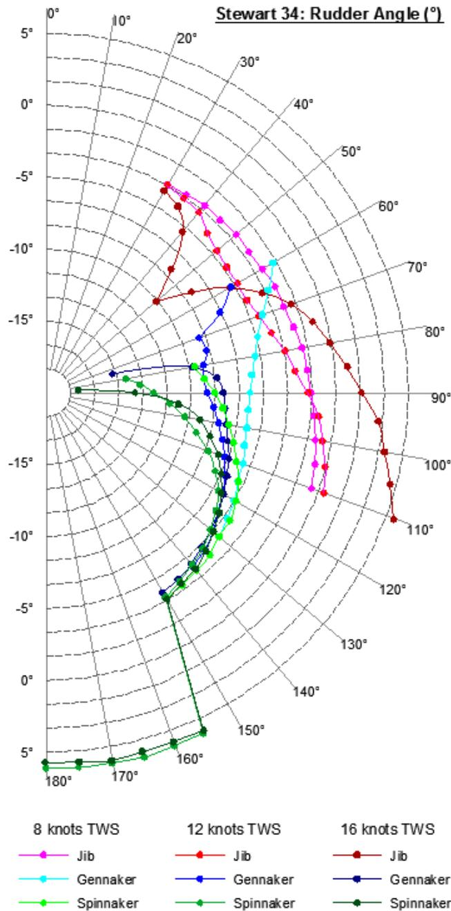
**Figure 70:** Stewart 34 FS-Equilibrium VPP: rudder angle (°).
