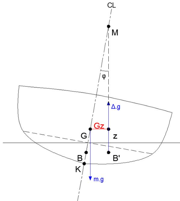
**Figure 56:** Transverse stability at small heel angles.
