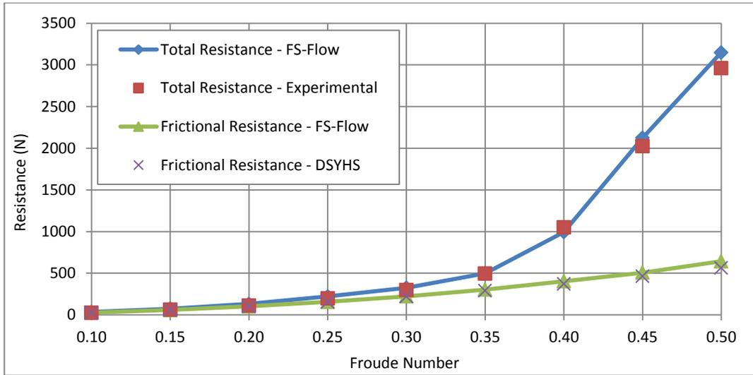
Figure 26: Bare hull upright resistance of the Sysser 62.
