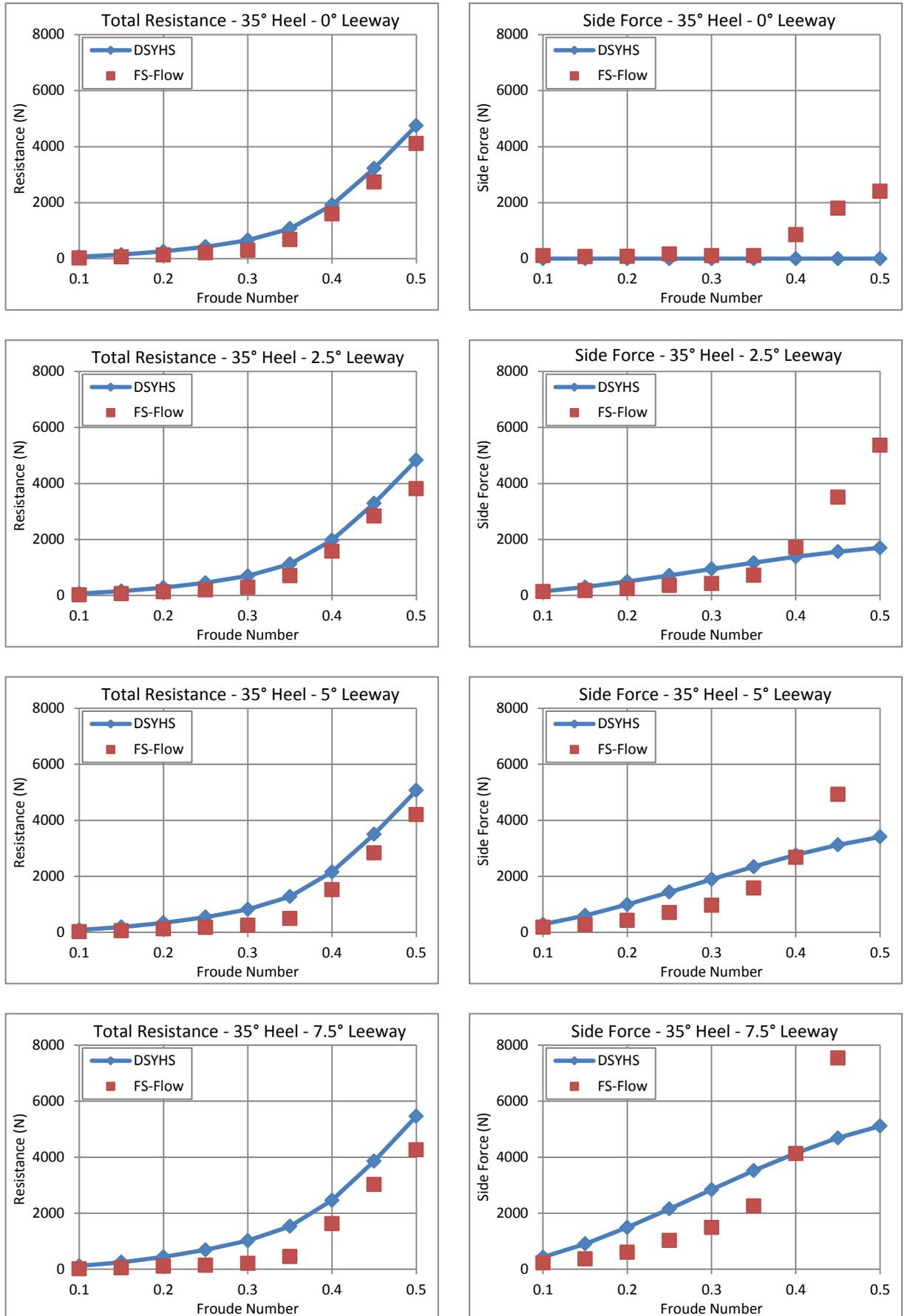
Figure 55: Stewart 34 hydrodynamic model: FS-Flow and DSYHS comparison, 35° Heel.
