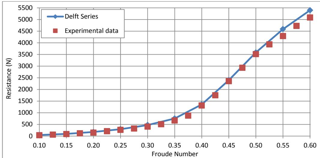
**Figure 7:** Upright total hull resistance, Sysser 62.
