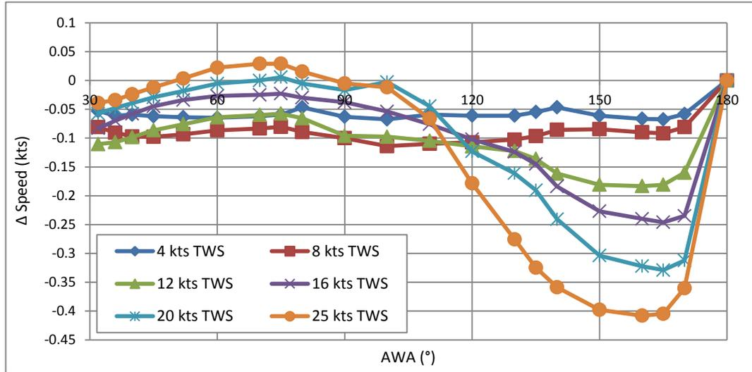
**Figure 61:** Speed difference (kts) between FS-Equilibrium and WinDesign.
