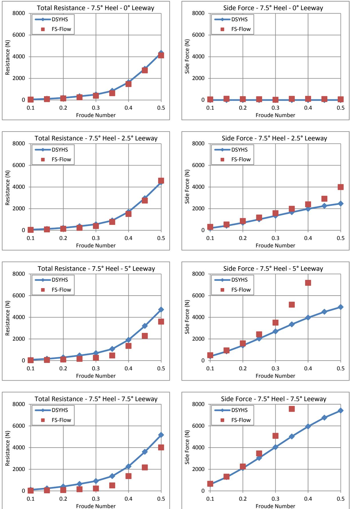
**Figure 51:** Stewart 34 hydrodynamic model: FS-Flow and DSYHS comparison, 7.5° Heel.
