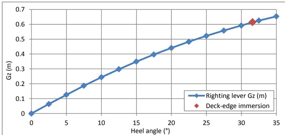
**Figure 59:** Gz curve of the Stewart 34 ascertained using Hydromax [8].
