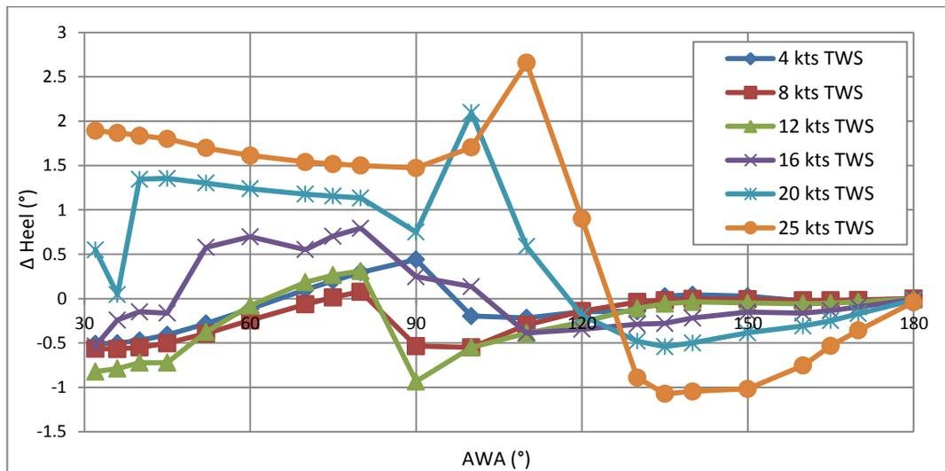
**Figure 62:** Heel difference (°) between FS-Equilibrium and WinDesign.
