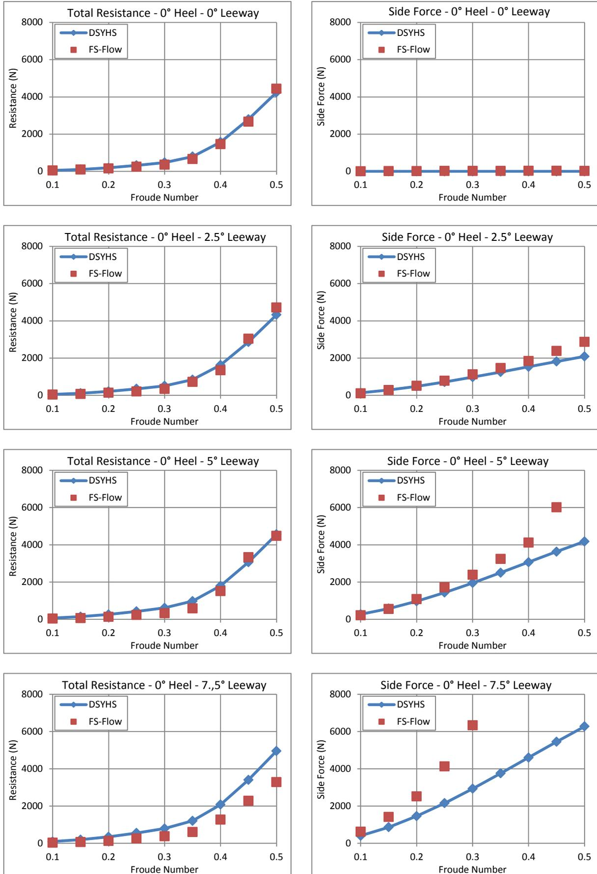
Figure 50: Stewart 34 hydrodynamic model: FS-Flow and DSYHS comparison, 0° Heel.
