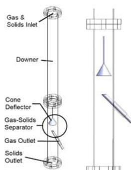
Figure 1 –Downer reactor Geometry (Huard et al, 2010)
